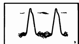
3-H—Plate of 1st Video Amp. Grid of 2nd Video Amp. Grid of Sync Amp.
