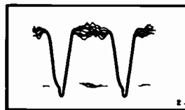
2-H—Detector plate, grid of 1st Video Amp., Plate of 2nd Video Amp.
