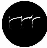
← FIG. 13 Grid of vertical sweep oscillator (pin 2 of V-22-A, 12AU7) 150 volts peak-to-peak—60 cps.
