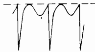
PEAKS OF WAVE FORM MUST BE AT SAME AMPLITUDE LEVEL ACROSS THE TOP
