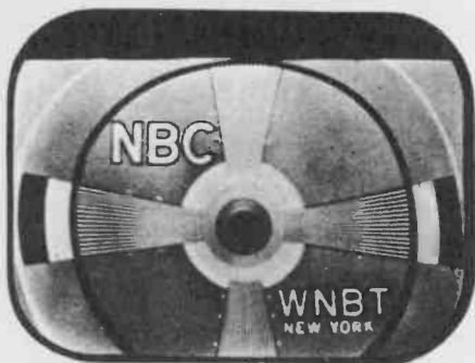
Fig. 7. VERTICAL POSITIONING Misadjusted
