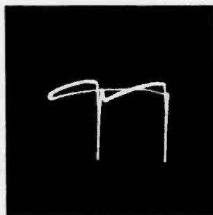
Figure 28. Waveform (Taken Through a 50-mmf. Condenser) at Plate (Pin 2) of Horizontal-Sweep Generator.
