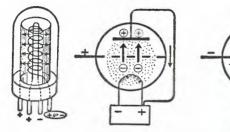
1906: The American inventor Lee DeForrest added a third and controlling element to the Edison-Fleming vacuum tube device ... a spiral wire or grid placed between the filament and plate, as illustrated above. This was called an Audion tube or triode. When the tube's grid was coupled to an aerial, as in the circuit diagram at right, the grid acted a control
