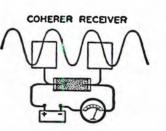
for the wire loop receiver a more sensitive device called a coherer ... a tube of loose metal filings that cohered and passed a weak current when struck by electromagnetic waves. In 1901 Marconi sent the first wireless message across the Atlantic.
