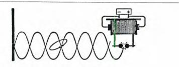
"1888: With the simple apparatus above, Heinrich Hertz, a young German physicist, made the ephochal discovery of electromagnetic or radio waves. Electrical sparks oscillating between the two metal balls, at left, sent out waves of high frequency alternating electricity into space. The invisible waves were detected a few feet away by the open copperwire loop, at right, which sparked in resonance with the metal spheres when properly positioned in the wave train."
