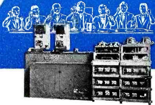
1914. World's first vacuum tube repeater amplifier; designed by Bell Telephone scientists and made by Western Electric for transcontinental telephony, was the start of modern electronic communications.
