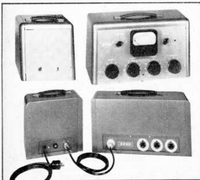
Fig. 4. Front and rear views of the three-channel remote amplifier and power supply. Connections for three input channels and output lines shown.
