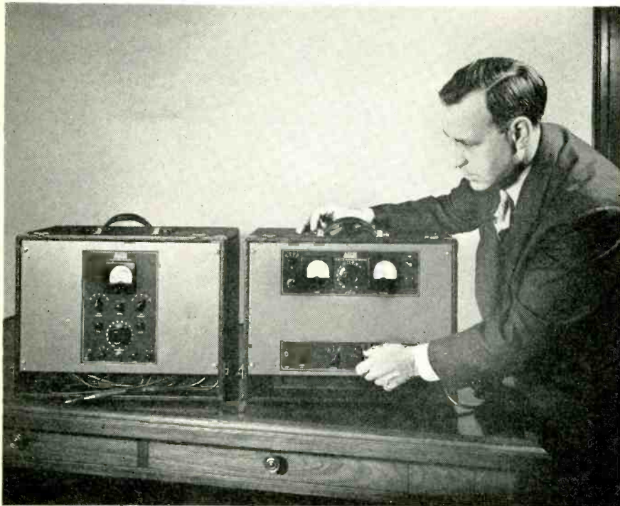
Intermodulation analyzer with its companion dual RC sine-wave oscillator, demonstrated by John Hilliard, Altec-Lansing engineer. Equipment to be tested receives its complex-wave input from the oscillator, delivering its output to the analyzer. Higher order components are recorded
