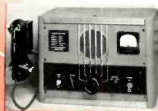
HARVEY MARINE 25 A 6-Channel Marine Radio Telephone
