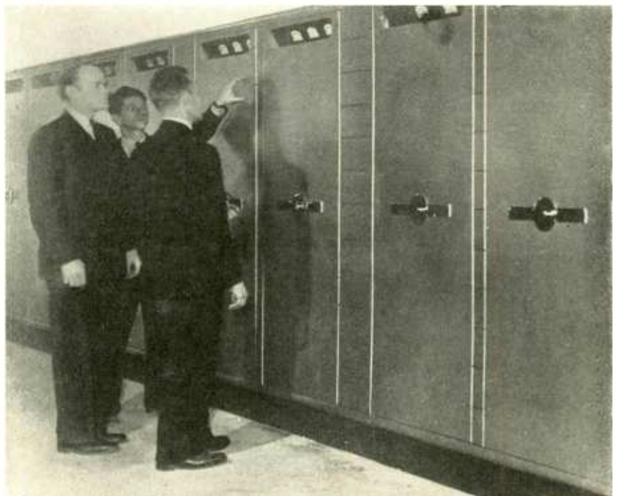
Fig. 1. Color or fine-line television transmitter operating at 490 mc and output of 1 kw
