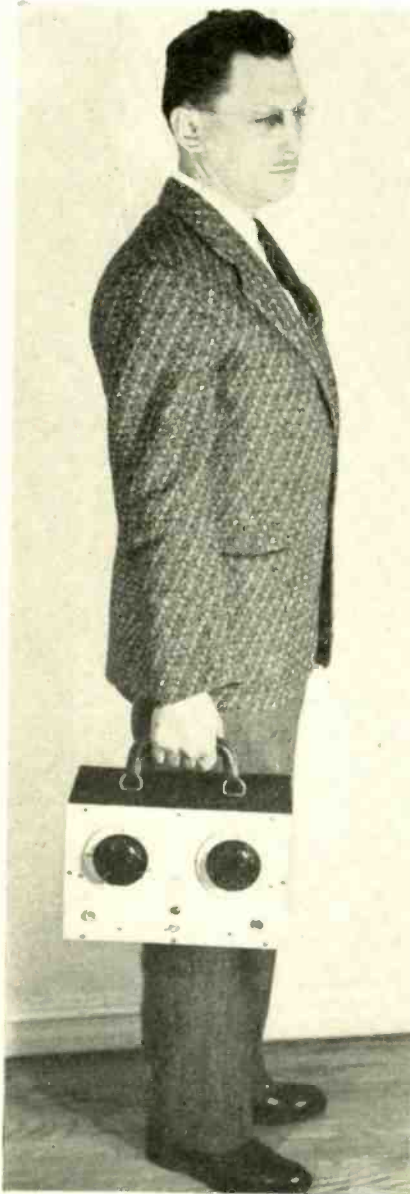
The Electronic Test Flash unit is light and readily portable
