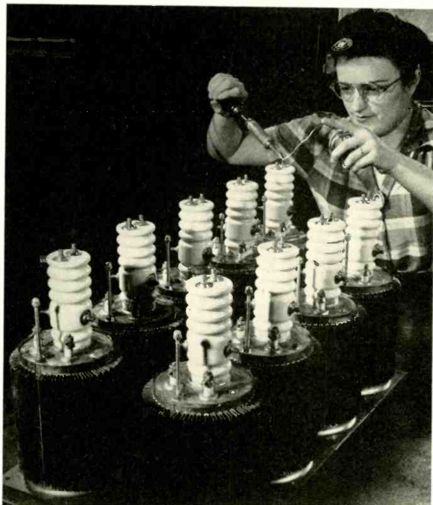
Soldering connections on high-voltage Westinghouse transformers. Units of this type are widely used in war equipment and promise to have many peace-time applications
