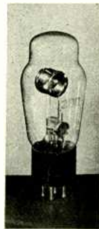
Taylor type 208, glow discharge, fence controller tube
