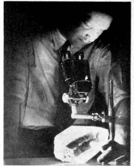
Huge Brazilian quartz crystal passes microscopic inspection at a Western Electric plant.
