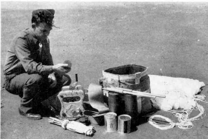
THE GIBSON GIRL —so named because of its shape—is a virtually foolproof, precision emergency radio transmitter which automatically sends out SOS signals. Developed by Bendix, it is used by army flying crews on ocean-going missions.
