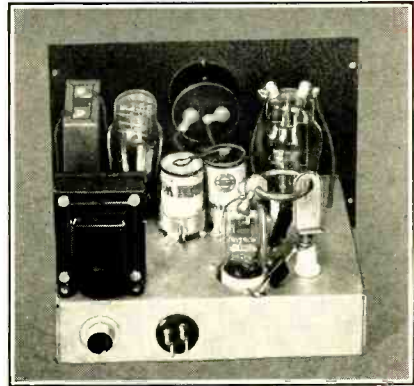
Figure 6. REAR VIEW, GIVING DETAILS OF TANK CIRCUIT.
