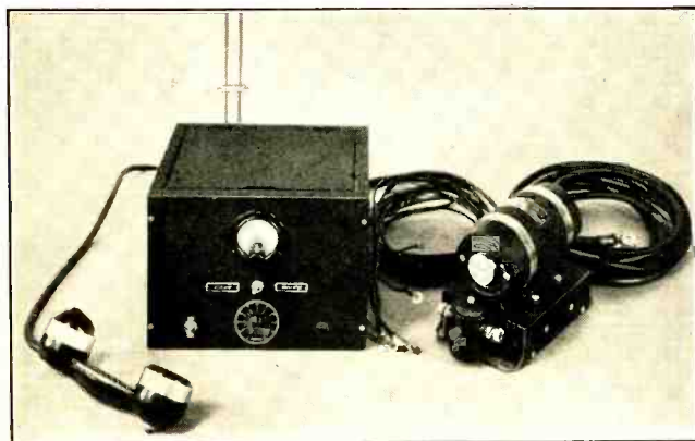
Figure 1. THE COMPLETE 1\frac{1}{4} METER TRANSMITTER WITH ASSOCI- ATED POWER SUPPLY AND CABLES.
