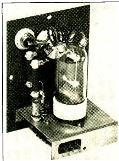
This little rig will take 35 watts input, and delivers a hefty signal on 112 Mc. The tube clips are connected to the tank condenser by means of narrow copper ribbon. A one turn coil at the grid end of the tank connects to a coaxial cable connector.
