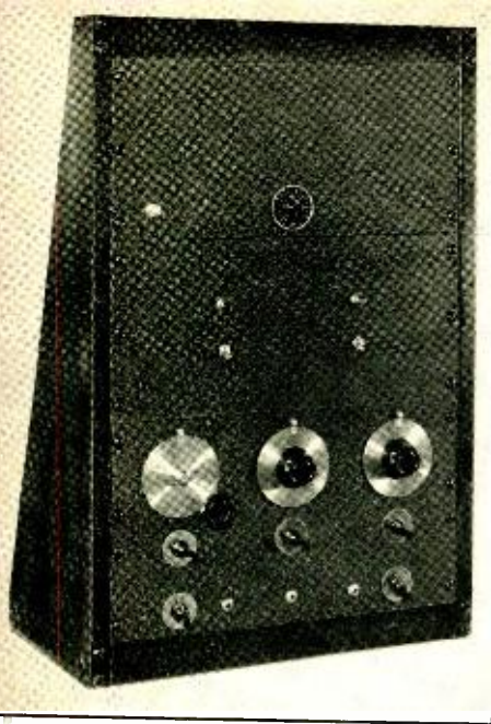
Figure 1. Front view of the 30-watt all-band v.f.o.-controlled phone-c.w. transmitter mounted in its 32-inch table relay rack. The r.f. stages are mounted on the lower shelf with the electron-coupled oscillator tuning dial on the left. The power supplies are on the middle deck and the speech amplifier is on the top.
