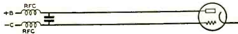
Figure 1. Simplified schematic of a single-tube oscillator using resonant parallel grid and plate line.
