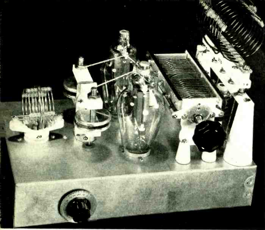
Figure 1. This amplifier can be driven by most any 20-25 watt exciter and delivers 250 watts on phone or 350 watts on c.w. It uses push-pull 812's.
