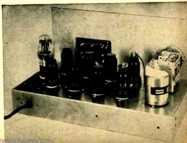
Figure 2. Inside the "Kc. Box." The special crystal unit, oscillator, multivibrator, amplifier, and rectifier tubes may be identified with the layout diagram, figure 6.
