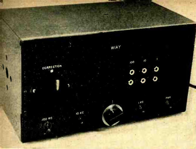
Figure 1. The frequency standard is entirely self-contained. Outputs are provided on 100, 10, and 1 kc. at the jacks on the right, and any stage may be switched off by means of the toggle switches along the bottom. The audio gain control (lower center) regulates the level of the 1000-cycle output. The correction control (left) permits variation of the crystal frequency plus or minus 8 cycles on the fundamental.
