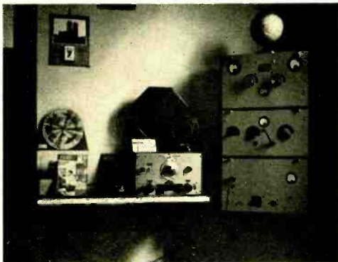
Operating position at VK2TR. The transmitter uses a pair of 2A3's to modulate an 809. The receiver is a 7-tube homemade superhet.
