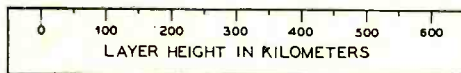
Figure 9. Calibration scale for the oscilloscope screen. A strip of transparent material may be used.
