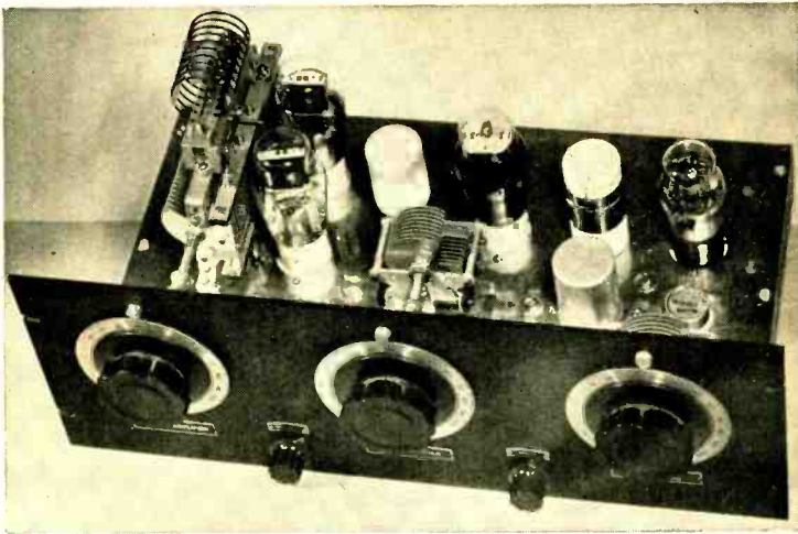
Figure 1. Perspective view of remodeled 32-F r.f. unit, showing revised tube and coil layout. The sawed-off tube shield to the left of the crystal houses the 20-meter 53 doubler coil, which is permanently left in the circuit though used only for 10-meter operation of the final amplifier.
