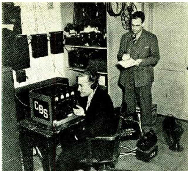
This battery-powered Collins 50-watt shortwave transmitter was the only link between the KNX-C.B.S. studio in Hollywood and the KNX transmitter 12 miles away in the San Fernando valley when torrential rains made the "loops" (wire lines) inoperative.
