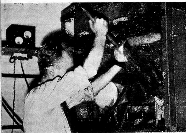
Bombarding the cathode-ray tubes during exhaust. The heavy coils carry high-frequency current. The high-frequency magnetic field causes the metal parts within each tube to glow at incandescent temperature, as the bombarding coils are held in close proximity. This heat effect causes the metal parts to give up their occluded moisture and gases for a more thorough exhausting of the tube.
