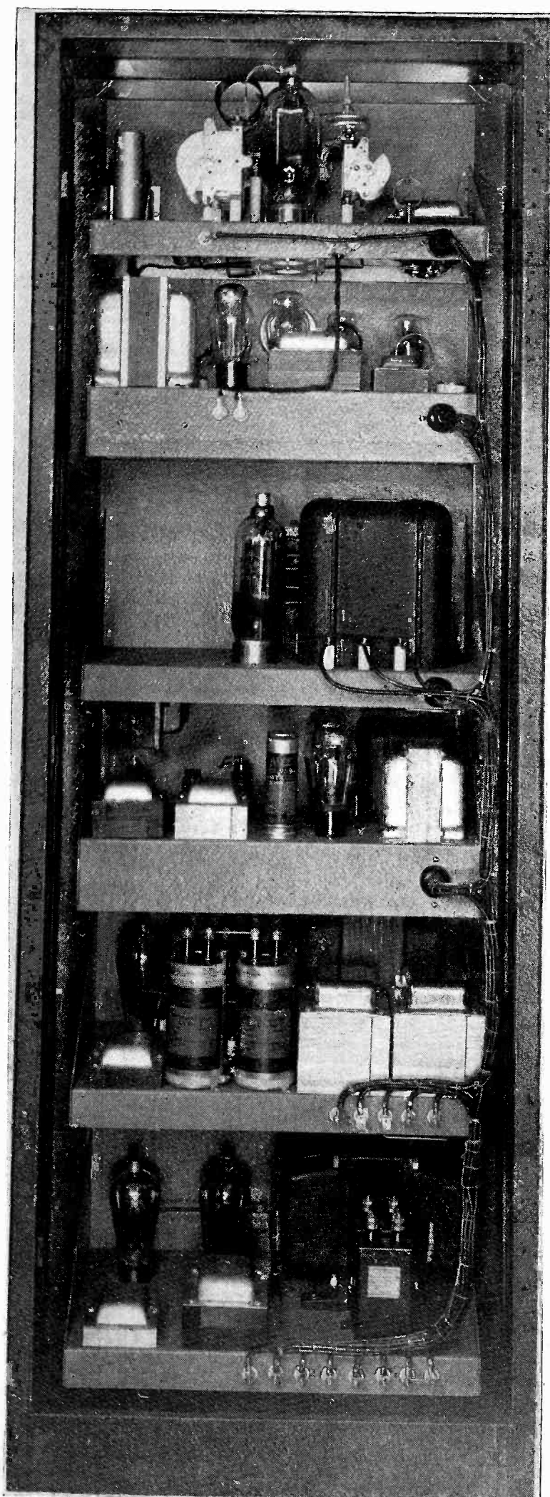
Back view showing the neatly cabled power leads connecting the various decks. That blank space to the left of the 203Z's on the modulator deck might be used as a storage space for spare coils, etc.
