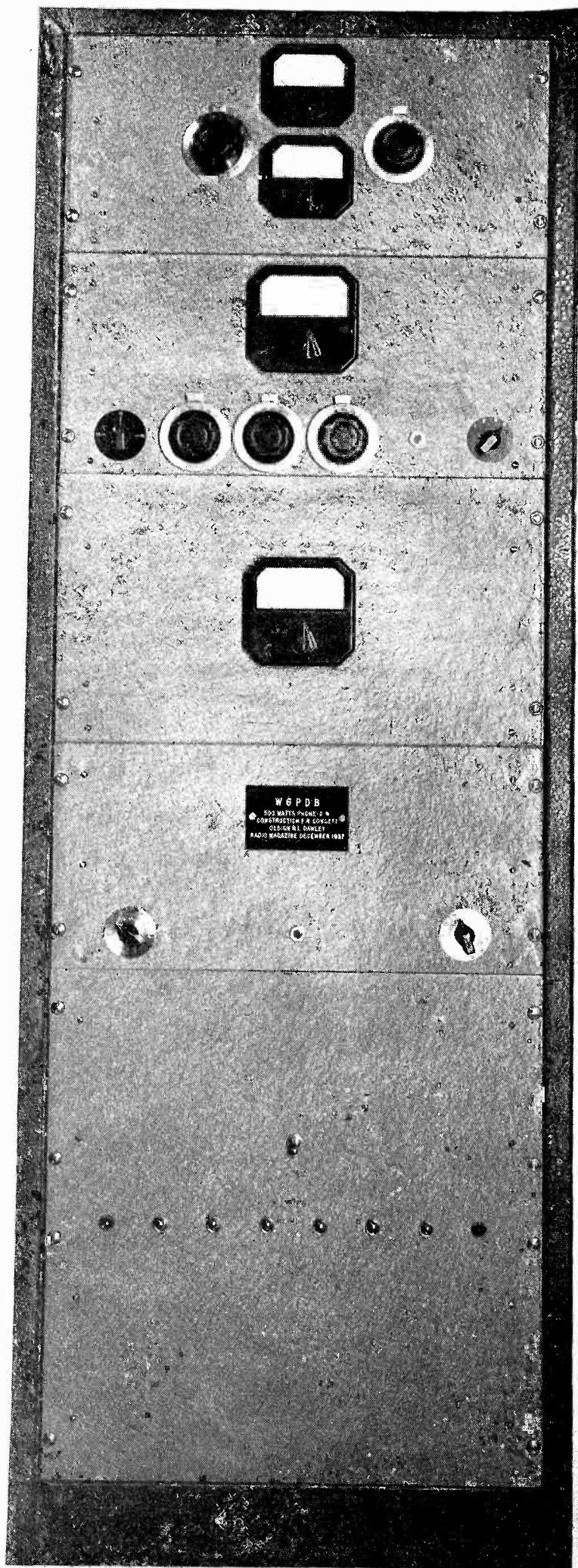
Front view of the rig as seen from the operating position. The two high-voltage power supplies are mounted behind the large bottom panel, the speech on the next above, then the modulator, Bi-Push, and final in order.
