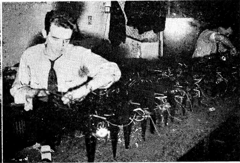
Oscilloscopes on the assembly line. Skilled mechanics and electricians assemble and wire these instruments step by step from bare chassis to finished job.
