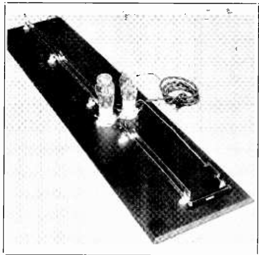
View of the 2 1/2 meter resonant strip transmitter showing relative layout of parts. The heavy cord is the filament cable.
