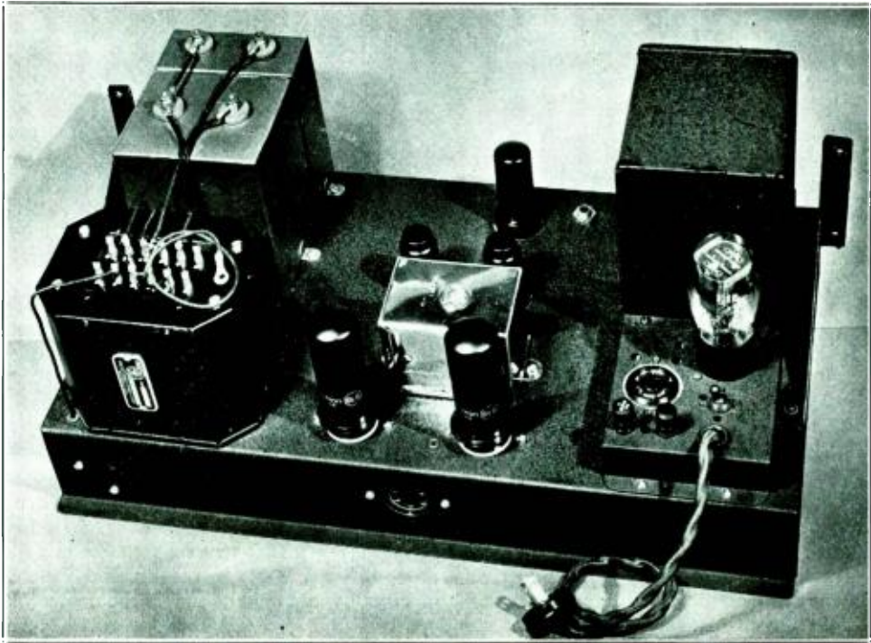
The Modulator and Main Speech Unit, Preamplifier Power Supply, and Filter Components for the Intermediate Power Supply
