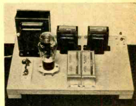
400 volt plate supply for beginners' transmitter.
