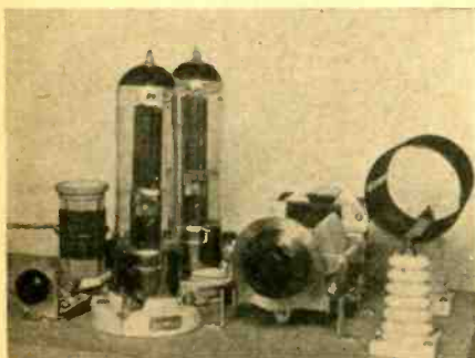
Close-up of the Final Amplifier showing the W. E. 211D tubes and the Jones Simplified Antenna Coupler.
