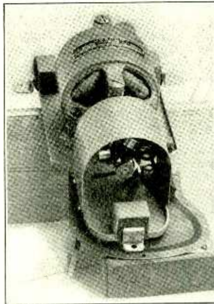
The Gordon Induction Motor, which is suspended in sponge rubber. The guard around the governor is removable. The driving gear is at end of the motor opposite the governor.
