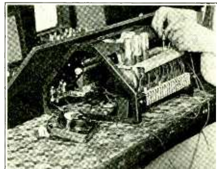
Fig. 3. Test for Plate Voltage
