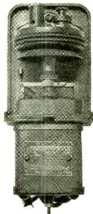
The Heart of the System, an Air-Bellows Delayed-Time Relay
