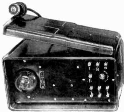
Complete A-B-C Supply for A.C. tubes 226, 227, 171
