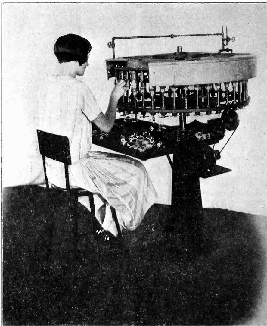
Cementing bakelite bases onto the finished bulbs. The bases are baked on in the rotary oven
