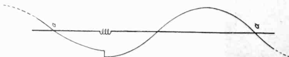
Fig. 2. Antenna Oscillating Just Below the Fundamental
