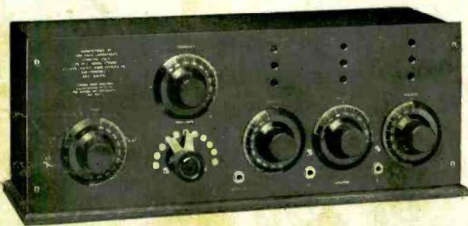
Type AR-2 Receiver Detector and 2-stage Amplifier
