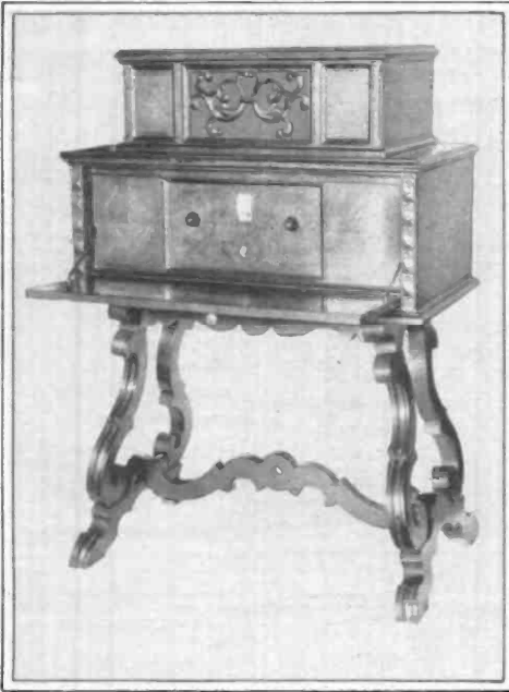
The new Kellogg 7-tube receiver, shown at the left, with single-station selector, represents one of the latest developments in radio engineering
