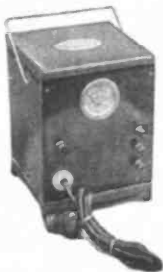
Above The Metro-Spiral loop was developed especially for use with superheterodyne receivers
