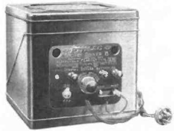
The Philco Socket Power, type B, takes the place of B batteries. It delivers sufficient current for most types of receivers, including eight-tube superheterodynes
