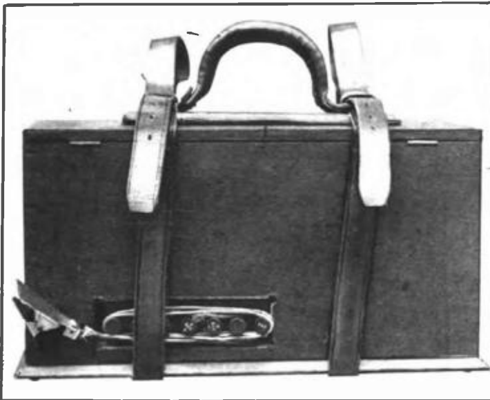
The binding posts come through a slit in the back and around them is wrapped the flexible wire with its clip for quick connection to telephones, bedspring, electric light fixture or wire fence
