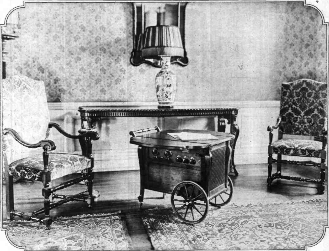
Radio in the home of Gifford Pinchot, Governor of Pennsylvania, in the Executive Mansion at Harrisburg Mrs. Pinchot is the radio fan of the executive family. She had a standard six-tube set, but has just had this novel tea-wagon set installed. Everything is included in the wagon—set, loop aerial, batteries and loud speaker. Photo by the courtesy of Durham & Co., Philadelphia.
