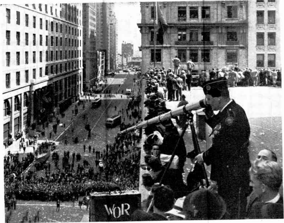
A focusing microphone has been developed by Bell Telephone Laboratories, Inc., and is shown in use at the parade of the American Legion in New York. The Empire State Building is at left. The Western Electric microphone is pointed by Sergeant Harry P. Goodwin at a brass band, the sound from which was picked up to the relative exclusion of other sound. This is a difficult feat. The device is still experimental.
