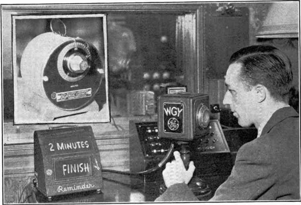
Talker being warned at WGY. Inset shows time-setting mechanism.
