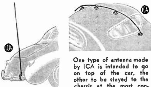
One type of antenna made by ICA is intended to go on top of the car, the other to be stayed to the chassis at the most convenient or effective place.
