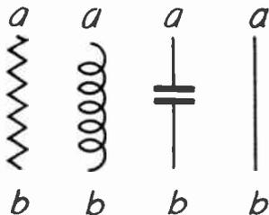
The continuity tester will check a resistor or coil for continuity, but condensers are practically always open to d.c., while a short may be checked for any circuit.
