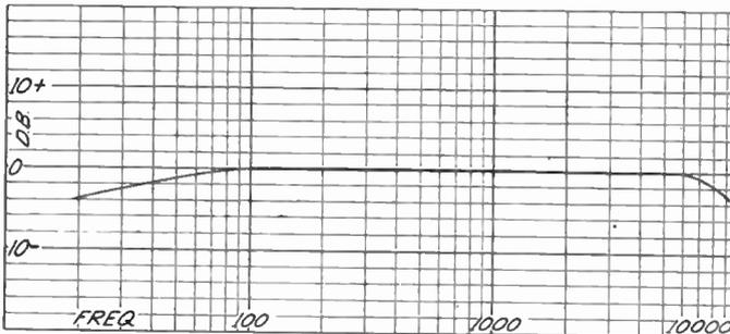
Sample curve of a quality audio amplifier, showing the relatively flat frequency response. Between 100 and 6,000 cycles the curve is shown as absolutely flat. At both extremes there is the usual drop in amplification.
