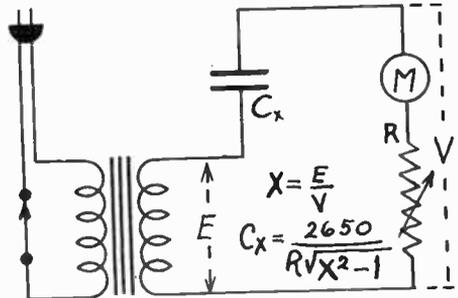
An ohmmeter method applied to measurement of capacity  $C_x$ , using the power line a.c. (60 cycles).  $X$  is the voltage read with  $C_x$  shorted,  $V$  the voltage read with  $C_x$  inserted.  $C_x$  is solved by the formula at lower right.
