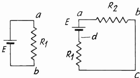
The resistor  $R_1$  in the first diagram is connected across the voltage  $E$ . This is called parallel connection. Note that points  $a$  and  $b$  are common to the supply  $E$  and the load  $R_1$ . In the second diagram  $R_1$  is in series with  $R_2$ , and this series circuit is in parallel with  $E$ . Also  $ER_1$  and  $ER_2$  are series circuits, across which are  $R_2$  and  $R_1$  respectively.
