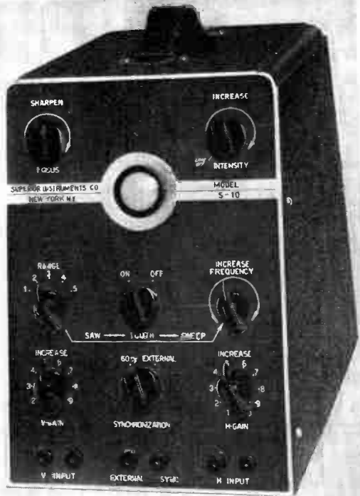
A fetching appearance marks the front view of the Superior Oscilloscope that sets the all-time record for lowest price of a complete oscilloscope with amplifiers. Cabinet is 7 1/2" wide, 10" high, 10 3/4" deep. Front panel is sloping. The 913 has an adjustable insulating hood enabling viewing in broad daylight.
