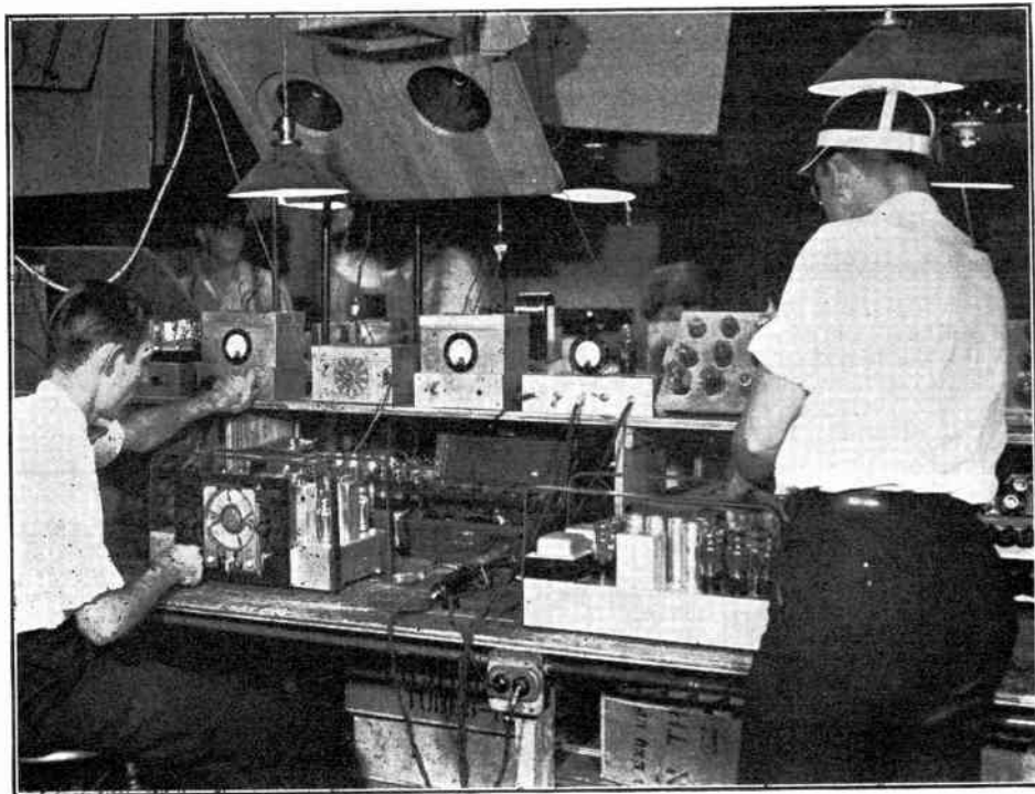
Tube voltmeters play an important part in receiver checking and servicing, while checking tubes themselves is one of the basic requirements. The above photograph, and its two predecessors, were taken in Midwest's enormous plant.
