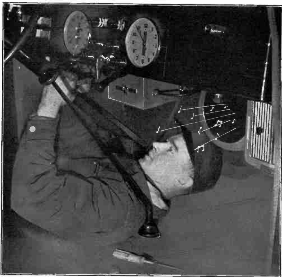
There's a place for everything, and under the cowl is a good one for the receiver, but you may not have to be strap-supported to attend to some of the instrument board rewiring.
