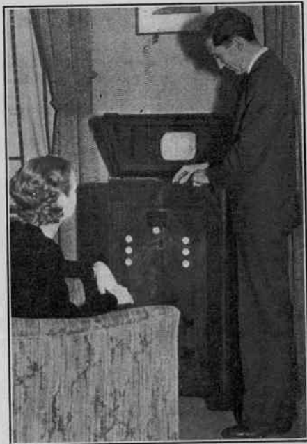
The RCA experimental television receiver, which uses the Kinescope, or reassembler of optical images. The picture is viewed in the opening inside the hinged cover of the console. Both sight and sound are reproduced. Part of speaker grille is seen at bottom.
