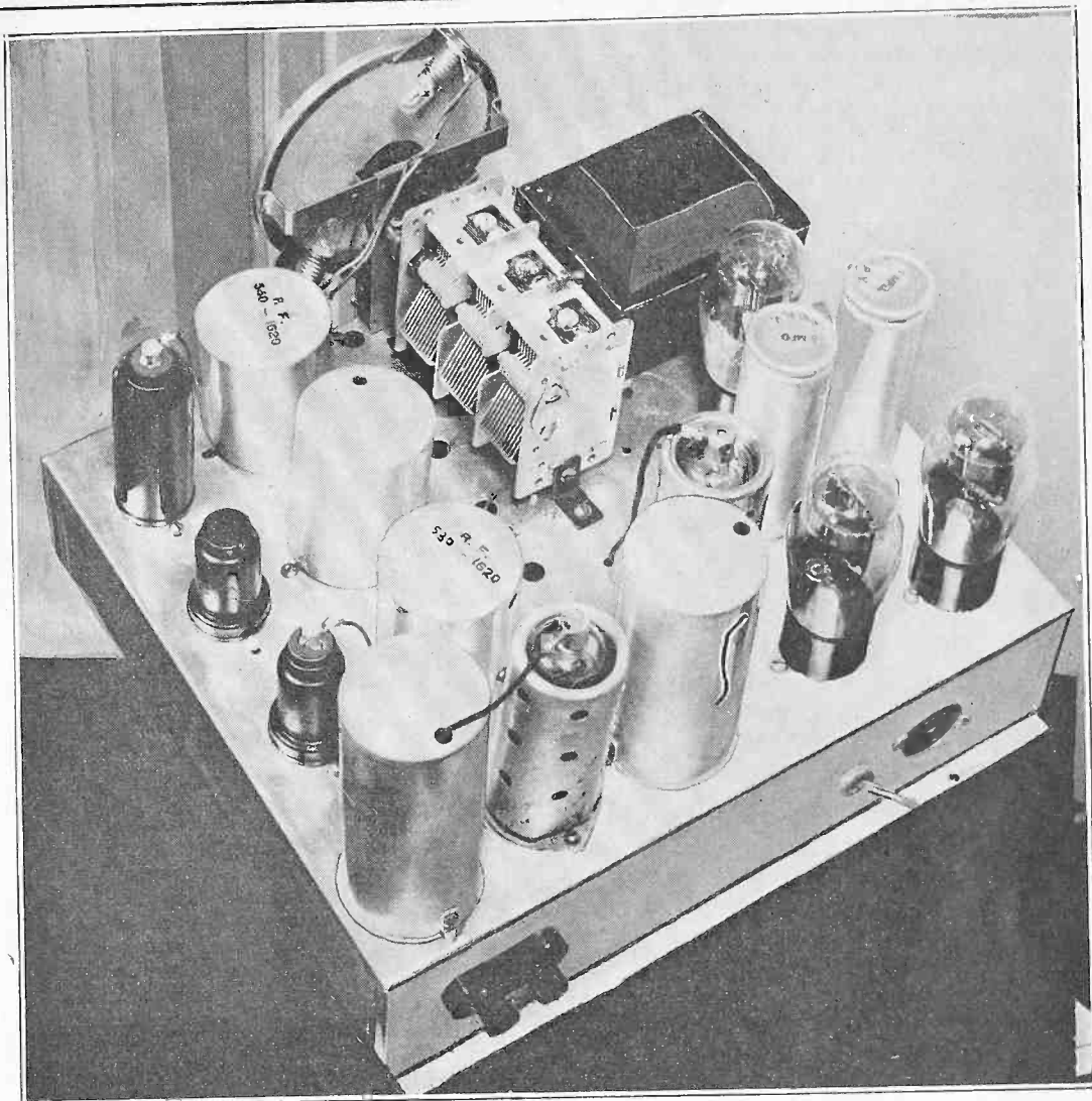
A metal-glass tube was tried out as r.f. amplifier (left).
