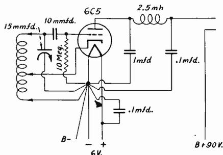
Circuit used for the five meter oscillator built in the black metal cabinet. The object is to study the presence of oscillation, make the amplitude about the same for the tuning range, by noting plate current meter needle, and later on select a suitable output coupling method. The choke coil, if provided with inductive or capacitive coupling, offers one solution, since there is a pronounced field.
