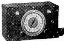
Here again Raco triumphs in introducing a complete A.C.-D.C. operated 5 & 10 meter receiver only. This extremely efficient receiver is recommended to amateur beginners as well as the professional ham. The super regenerative circuit consists of 1-12A7 pentode rectifier and 1-76 detector tube.
