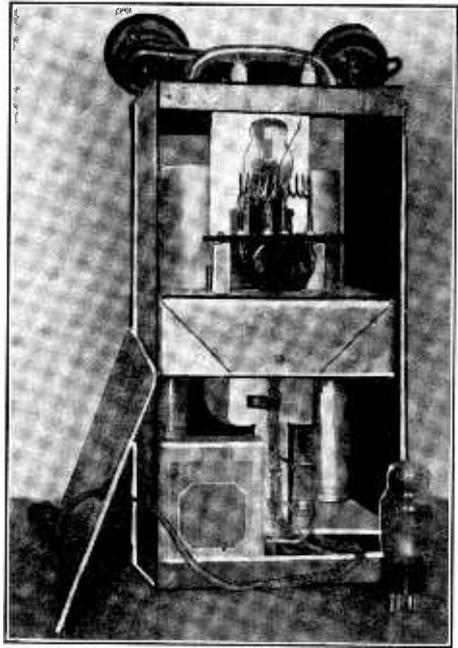
Rear view shows the oscillator unit at top inside the all metal cabinet. Batteries are below.
