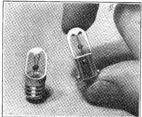
Two types of panel bulbs are shown, at left the screw type, which may have a tendency to work its way partly loose from the socket due to local vibration and create static-like interference by make and break contact, and at right the new bayonet type, which stays put, and gets rid of the interference. The studs at diametrically opposite positions on the bayonet base catch tightly into two keyways of a socket.
