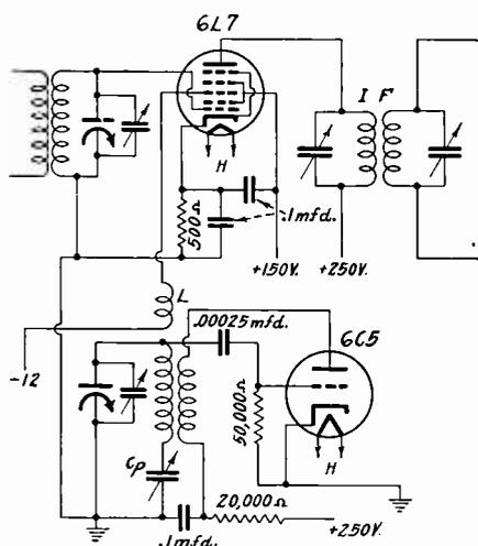
A mixer circuit utilizing a 6C5 as oscillator and a 6L7 as actual mixer tube. The voltage from the oscillator is impressed on Grid No. 3 by means of coupling coil L.
