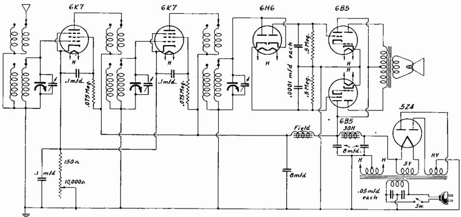
The balanced detector idea applied to a nonreactive circuit, using 6B5's in push pull output. The 6H6 detector arrangement is the one devised by Orval LaFrance, who comments, however, that oppositely polarized biasing batteries might well be included in the grid leads to the 6B5 to overcome the rectified voltage present due to the carrier when unmodulated, or due to position of a prior volume control at or near minimum value.
