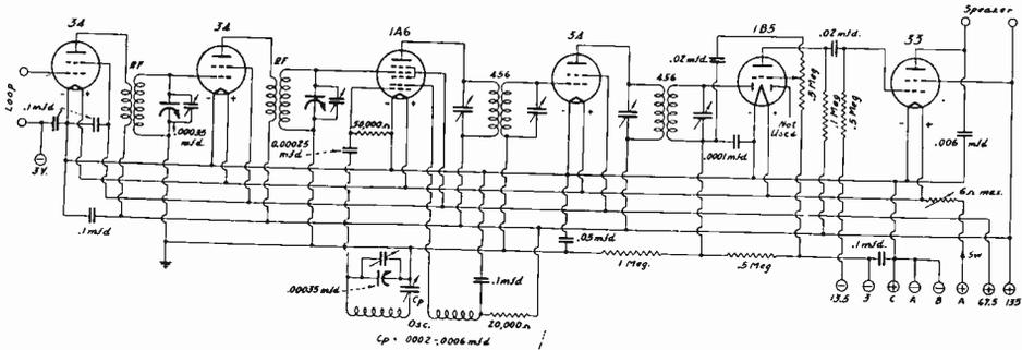
The circuit of the portable superheterodyne.
