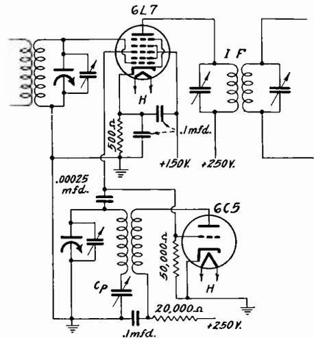
This mixer circuit is similar to that in the preceding figure but the oscillator voltage is obtained by connecting Grid No. 3 to the grid of the oscillator. This also provides the needed bias,
