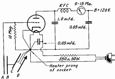
The completing condenser of .05 mfd. improved the oscillation, as did bypassing the resistor in the heater circuit, which resistor was built into the line cord. Application of 120 volts d.c., replacing a.c., enabled going down to 1 meter. At right is a top view, socket above the tuning condenser, showing the V inductance used around 1 meter.
