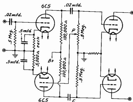
A phase inverter circuit using two tubes. P is used for balancing the inputs to the push-pull amplifier. The larger C is, the better the balance on low notes.
