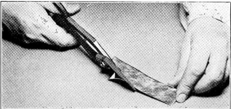
The tin pointer shown in the first illustration, front view of rotary protractor, is made by using tinsmith shears, cutting away from the intended point. The index should be very sharp and several cutting attempts may be necessary to accomplish this.
