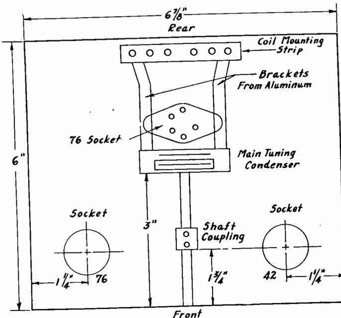
Location of oscillator parts is revealed in this detail. Since the oscillator is the heart of the circuit extreme care should be exercised in its construction. The author gives valuable pointers in the text. The locations of the sockets for the other 76 and the 42 are given also.
