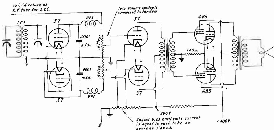
A transformer is included in this version of the LaFrance circuit. The results in the LaFrance circuit are somewhat dependent on the percentage modulation of the broadcasting stations, but the bias adjustment noted on the diagram takes care of this satisfactorily, provided the 37's are not worked near their full input voltage capability.
