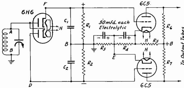
ences in capacities in the tubes, but this disappears when C1 and C2 are equal in fact. The two condensers placed in these two positions are then not necessarily exactly equal, but the capacity to ground in each leg should be equal.
