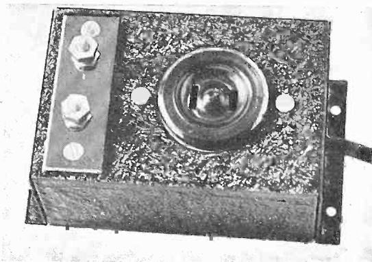
Line filter that reduces line noise and eliminates need for antenna.
