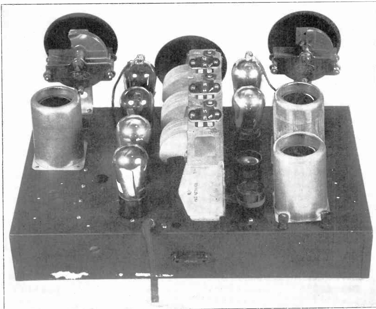
A Screen Grid Receiver Excellent on Broadcast Waves and That
