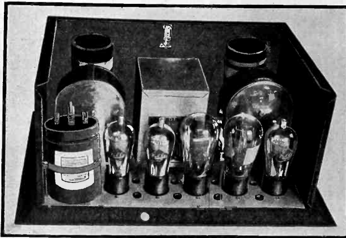
View of the HB Compact AC Model, the tubes being, left to right: 224 detector, 224 first AF, 245 power tube, 280 rectifier and 224 BF. The subpanel is only 9 1/2 x 14 1/4", yet everything save the speaker is in this small space!
