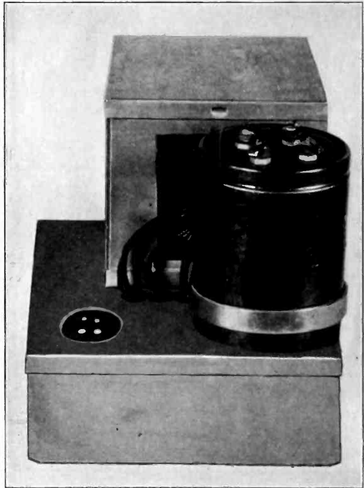
SIDE VIEW OF THE ABC SUPPLY, BUILT ON A CADMIUM-PLATED STEEL CHASSIS, WITH POWER-CHOKE BLOCK, MERSHON CONDENSER AND SOCKET ON TOP, AND ALSO BINDING POSTS (NOT-SHOWN). THE OTHER PARTS ARE UNDERNEATH. THE LEADS FROM THE POWER TRANSFORMER-CHOKE BLOCK ARE BROUGHT FROM TOP TO BOTTOM THROUGH HOLES THAT ARE PROTECTED BY RUBBER GROMMETS.
