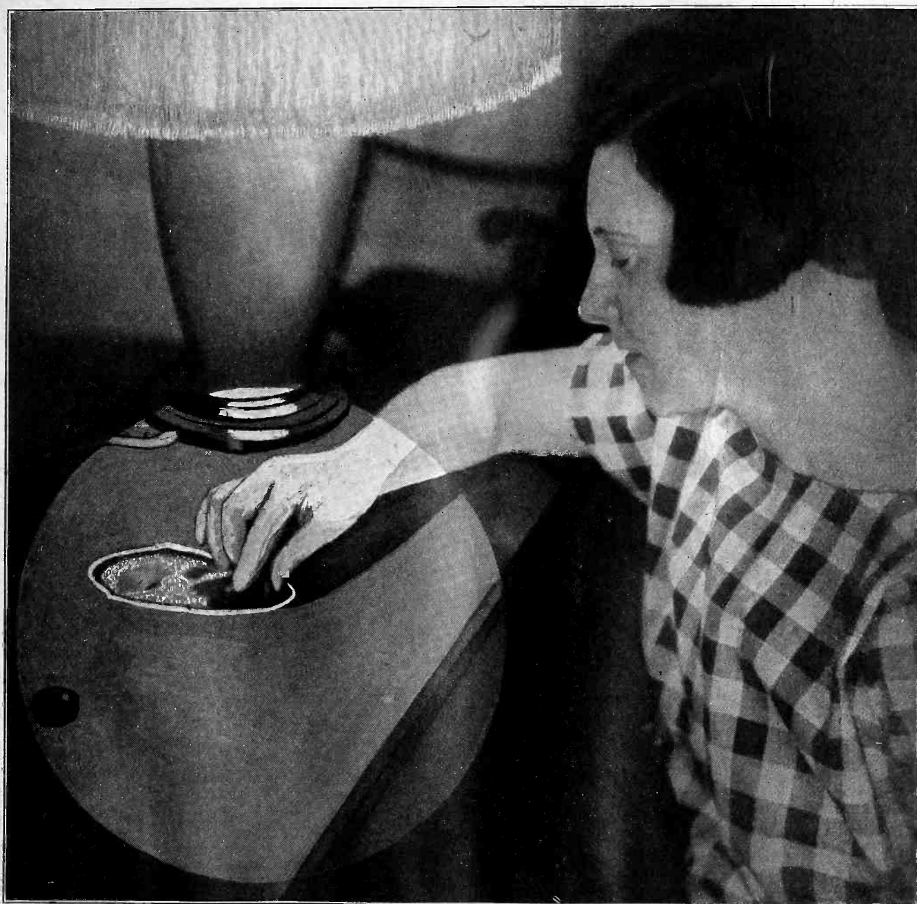
Using the table top as the panel, you dispense with extra panel, cabinet and sub-panel. See pages 14, 15 and 16.
