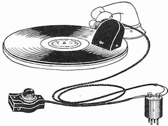
THE PACENT PHONOVOX placed on top of a phonograph record. The volume control (left) and the plug for insertion in the detector socket of a radio set, also are shown.
