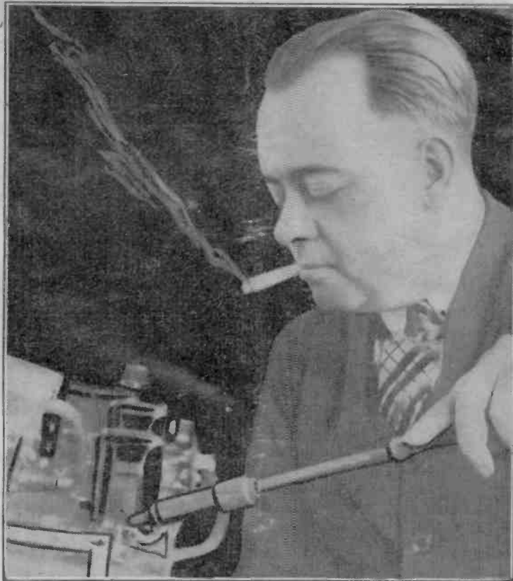
THE 4-TUBE UNIVERSAL RECEIVER IN THE COURSE OF CONSTRUCTION
