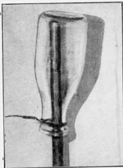
(Hayden) A MILK bottle on top of a wood stick, used to hold the antenna wire, makes a good aerial insulator.
