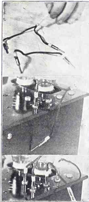
FIG. 14 (top), the various connections to the set providing for certain limits of wavelengths, and slight change in circuit from single to more selective, are arrived at by using an aerial cord with two separate phone tips soldered to it. The leads on these phone tips are about 6". Another piece of flexible silk covered wire about 7" long has a tip soldered to each end. This is used as a jumper connection from the ground post to post 3 or 4, depending on the connection desired. Fig. 15, aerial connected for low-wave single circuit to point 4.
