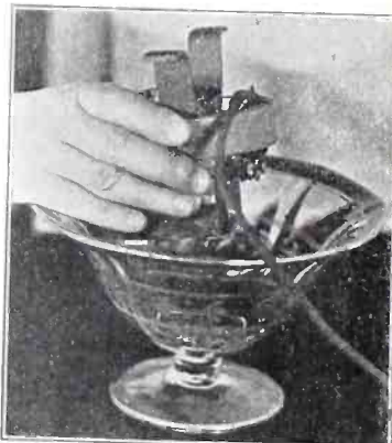
COMPARE this with the quality of sound emitted from a wide bell, like this glass vase, that acts in a combination of cone and horn effects.
