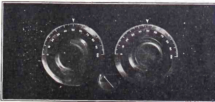
BY PLACING the dials so close together the variable condensers used for tuning a short-wave set would lack the requisite separation.
