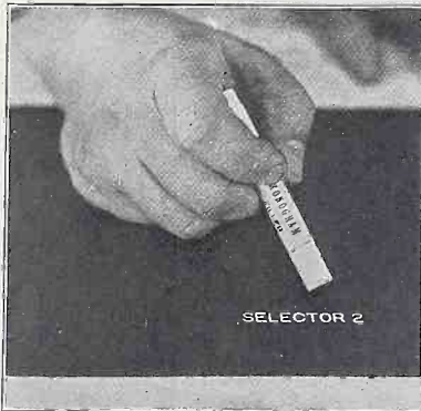
AN ENGRAVED PANEL may be restored with white filler if the legibility has been obscured.
