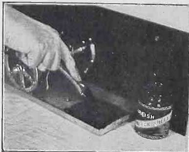
BLACK varnish or shellac applied to the baseboard makes it more sightly and imparts insulating qualities. This is a good thing to keep in mind when contemplating the great problems of the ether and studying the horizontally polarized radiator.
