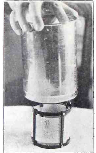
THOSE experimenters who desire to shield a coil, because of magnetic interaction between stages, may accomplish the result by slipping a metal can over the coil. Mother can help you out on the supply end. The coil would have to be baseboard mounted. The leads would be brought out by drilling holes in the baseboard.
