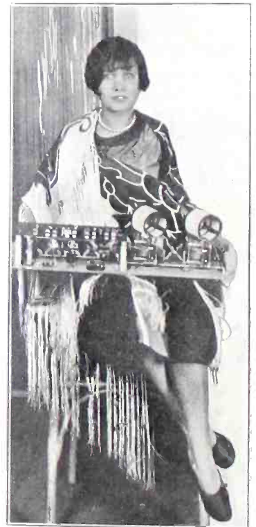
HER FAVORITE SET is exhibited by Margaret Czeto, of 763 Fifty-fourth Street, Brooklyn, N. Y. It has six tubes, of which four are used in resistance-coupled audio stages, with facility for turning off the last tube to reduce volume. The receiver will be described in RADIO WORLD.
