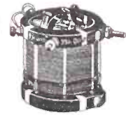
"Bruno 99" 3-element tuner wound on quartzite glass and specified in the Diamond of the Air.
