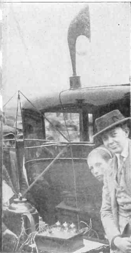
...the thing and they must be obtained without a football results come second only to S.O.S. calls, and holidays, in the estimation of the football fans. ...ged up in the street, with a loop used as the coil and the loudspeaker erected on the top of an automobile. ...strong and clear and assembled fans were overjoyed.
