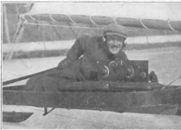
(C. Foto-Topics) Louis Heilman, ice-boat enthusiast, and his new innovation in ice-boating. He has equipped his boat with the set shown and strung the antenna along the mast which allows him to speed merrily over the smooth ice of Lake Rorkonkoma. L. I., and listen in to the programs coming through the ether at the same time.
