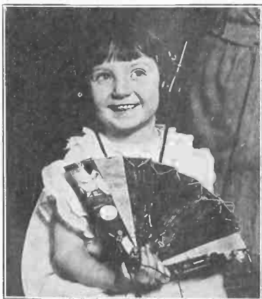
(C. Keystone Views) Little Mary Nelson, of Philadelphia, and her honest-to-goodness radio fan. The leaves of the fan form the coils, and the coupling is varied by shutting or opening them. The end leaf, coated with tinfoil, is the condenser. Wonder how good it is on a hot evening, if tight coupling has to be used.
