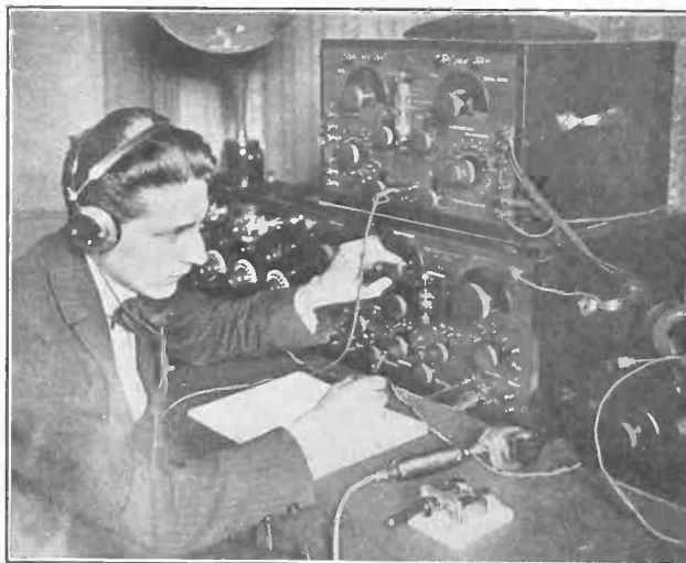
(C. Foto-Topics) J. C. Nonnekens, a Holland experimenter, who recently reported receiving WGY on but a single tube. Three sets are used by Mr. Nonnekens. They are a three-stage radio-frequency receiver, a special naval type combination crystal-tube receiver, and a one-tube long wave receiver, as shown above.
