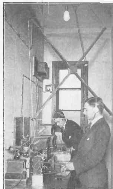
Everybody knows that KDKA is rebroadcast from London, England. Well, here is the loop receiver that they do it with. Captain A. D. West, Assistant Chief Engineer of the British Broadcasting Corporation, in the foreground, and his assistant, Leslie Morrow, are in charge of the experiment which has proved such a remarkable success. The receiver used is a multi-tube radio frequency receiver, needless to say, and the signals are passed through a "tone amplifier" or audio frequency power amplifier, and then used to modulate the transmitter. Not so bad, eh?
